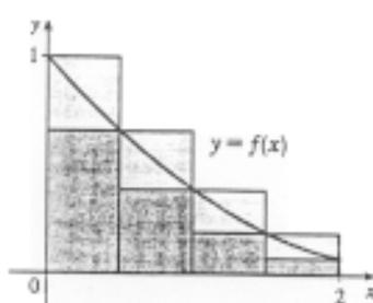
The diagram shows that  $L_4 > T_4 > \int_0^2 f(x) dx > R_4$ , and it appears that  $M_4$  is a bit less than  $\int_0^2 f(x) dx$ . In fact, for any function that is concave upward, it can be shown that
