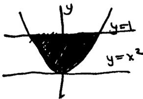
cross section of tank has length  $2x = 2\sqrt{y}$
