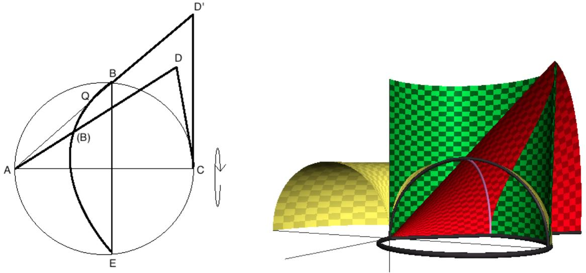
The surface of the cone described by the rotation of  $ACD$  will meet the curve created by the intersection of the half-cylinder and the half-torus (described by the rotating half-circle on  $AC$ ) at a point  $P$ . Put another way,  $P$  is the point at which the surface of the cone intersects the curve created by the intersection of the half-cylinder and the half-torus.
