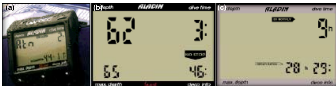
Figure 5: Wrist mounted diving computer manufactured by UWATEC. (a) The dive computer unit. (b) During a dive the computer displays current depth (62 feet), maximum depth (65 feet), time under (3 minutes) and time remaining (46 minutes). (c) After the dive the computer displays the number of hours before the diver can fly (9 hours) and the time required to completely eliminate dissolved nitrogen from the blood (28 hours, 29 minutes).
