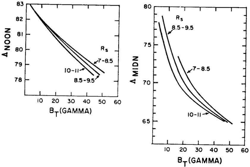
Fig. 46. Latitude of the earth intersection of the noon and midnight limit of "closed" field lines [12] as a function of the tail field intensity  $B_T$  and for different intervals of stand-off distance  $R_s$ , for the Mead-Williams model
