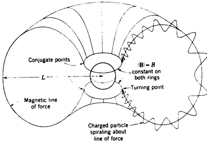
FIGURE 7 Motion of a charged particle in the geomagnetic field (Space Science, C. A. Londquist ed., 1966, McGraw-Hill, N. Y. ).
