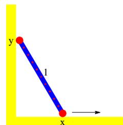
In reality, the ladder breaks away from the wall. One can calculate the force of the ladder to the wall. The force becomes zero at the **break-away angle**  $\theta = \arcsin((2v^2/(3g))^{2/3})$ , where  $g$  is the gravitational acceleration and  $v = x'$  is the velocity.
