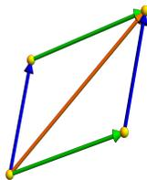
FIGURE 2. The addition of two vectors produces a vector in which one goes first along the first vector and the along the second vector. Doing this in the two possible orders produces a parallelogram.
