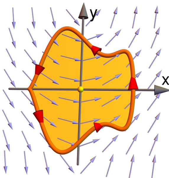
FIGURE 2. If  $\vec{F}$  is a gradient field, then Green's theorem can be understood more easily. The boundary line integral is zero because of the fundamental theorem of line integrals. The double integral is zero because the curl is zero for a gradient field.
