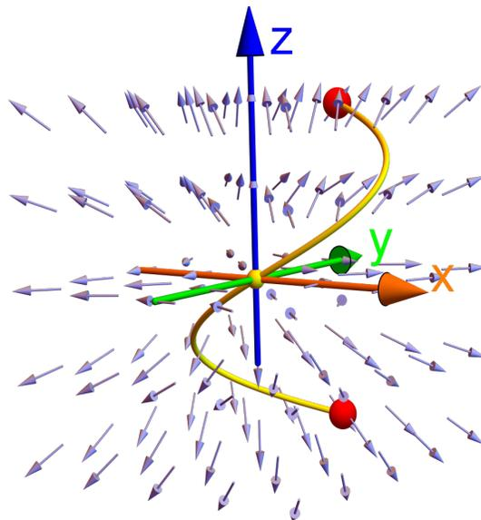
FIGURE 1. We see the gradient field  $\vec{F}(x, y, z) = \langle y, x, z \rangle$ . It has the potential  $f(x, y, z) = xy + z^2/2$ . Instead of computing the line integral along the path  $\vec{r}(t)$  from  $A$  to  $B$ , we can just evaluate the function at  $A$  and  $B$  and form  $f(B) - f(A)$ .
